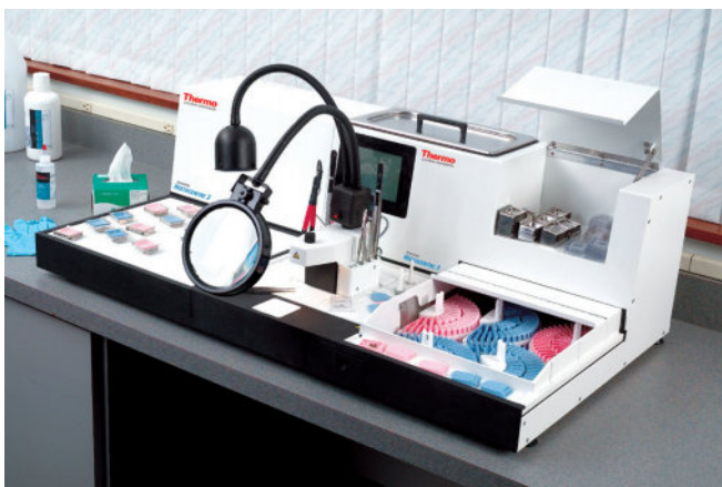
FIGURE 2.4 ♦ Tissue embedding centre, Model Histocentre (Photograph courtesy of Thermo Shandon, UK through Towa Optics (India) Pvt. Ltd., Delhi).
