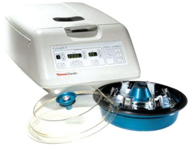
FIGURE 39.2 ♦ Cytopsin used for making smears in cases with small volume of fluid (Photograph courtesy of Thermo Shandon, UK through Towa Optics India Pvt. Ltd., Delhi).
