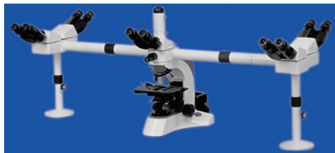
FIGURE 1.3 ♦ A penta-headed light microscope, for simultaneous use by one primary user and 4 other users seated nearby.
