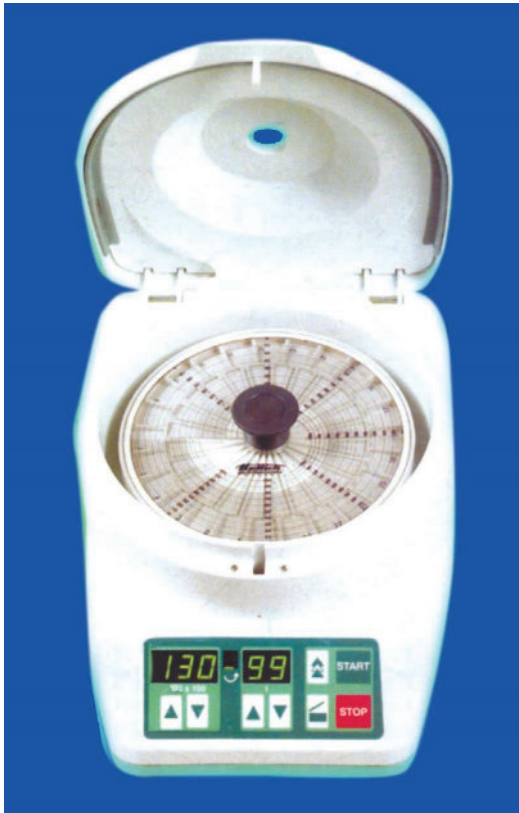
FIGURE 52.3 ♦ Microhaematocrit method for PCV. Haematocrit 20 model (Photograph courtesy of Hetlich, Germany through Global Medical System, Delhi).
