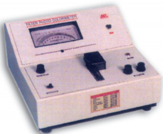
FIGURE 47.1 ◆ Photoelectric colorimeter used for taking reading of haemoglobin in cyanmethaemoglobin method and oxyhaemoglobin method. (Photograph courtesy of Max Electronics India, Chandigarh).
