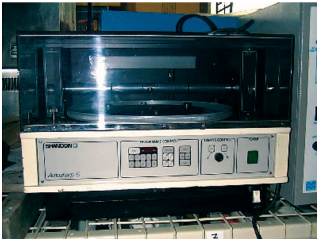
FIGURE 2.7 ♦ Automatic knife sharpener, Model Shandon Autosharp 5 (Photograph courtesy of Thermo Shandon, UK through Towa Optics India Pvt. Ltd., Delhi).
